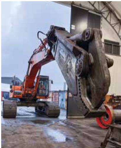
Amix Marine Services repairing the shear which is used for demolition.
